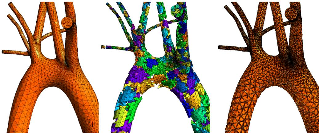
Figure 1: Graphical example of the three evaluation strategies in the context of an aorta simulation showing the globally assembled system (left), local elemental system (right) and a partitioning of the mesh to create a hybridized system (center).
